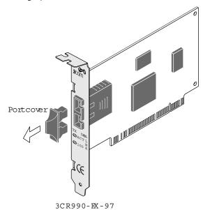
The 3CR990-FX-97 NIC provides these features for supported IP and IPX environments:
